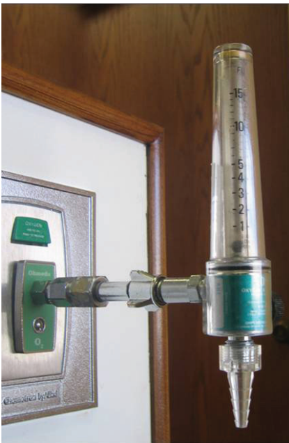
Figure 3. Better Design of Spigot Using Clear Attachment
