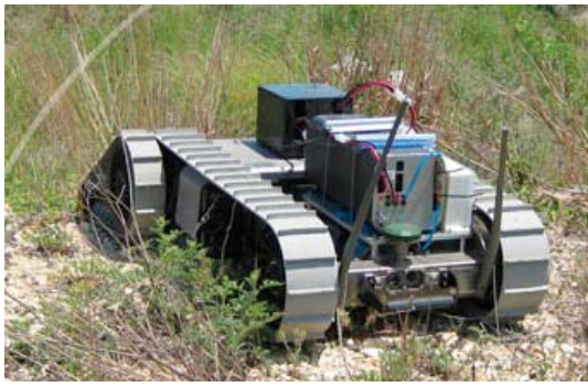
Figure 8. Adaptive Materials' Fuel Cell-Powered Mobile Robot
